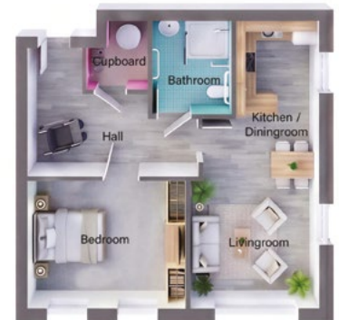
Typical wheelchair accessible 1-bedroom apartment
