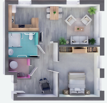
Typical Wheelchair Accessible 1 Bedroom Apartment
